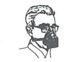
good seal on any face. To check dust seal of facepiece remove filter holder in accordance with paragraph three, place palm of hand over hole and inhale gently. If the respirator is properly fitted, the wearer should not be able to breathe thru the respirator or feel any inward leakage of air around the edges of facepiece.
